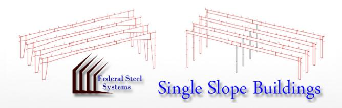
Federal Steel Systems' Single Slope frame design, commonly known as a "shed roof", can be designed as a clear span or multi-span frame. This frame design is commonly used for building additions, loafing sheds, hay storage, and equipment storage. Federal Steel Systems can also incorporate this design when site conditions dictate that roof drainage can only flow in one direction.
